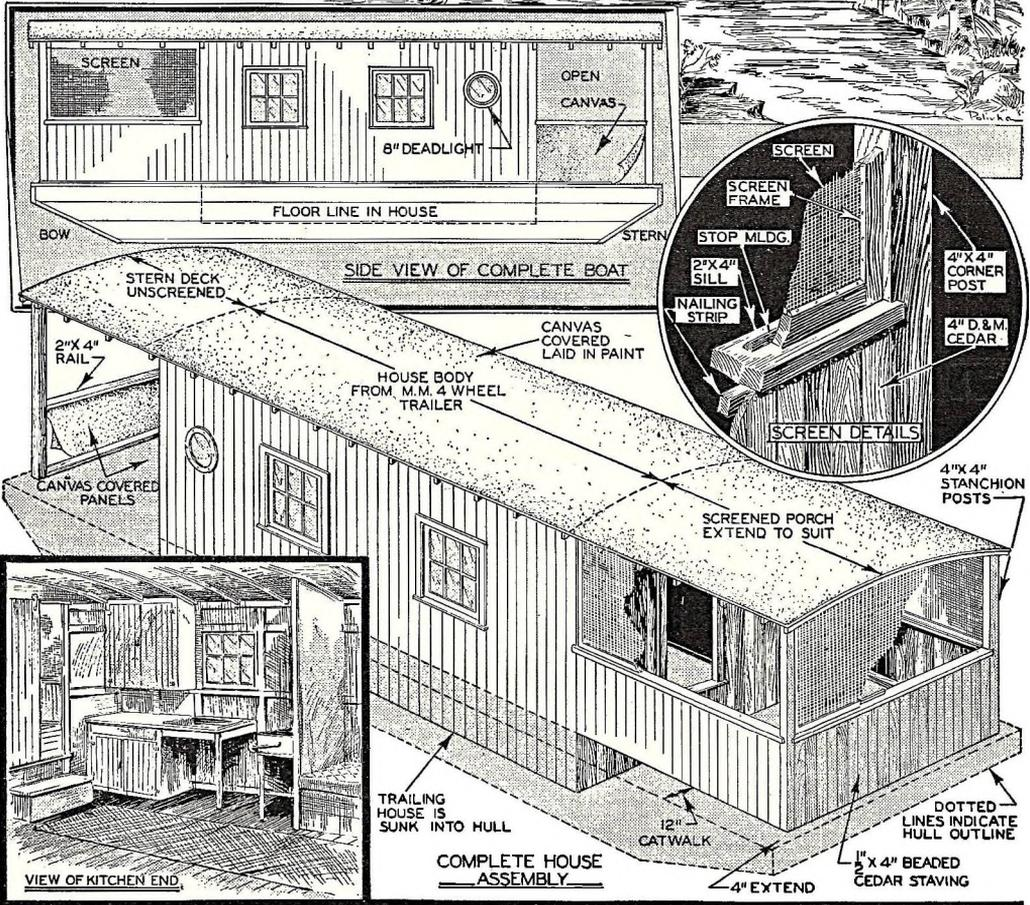
The thumb nail sketches show how attractive the interior can be made. The catwalk space of 12 ins. around the cabin is necessary for handling the boat. Elevation and isometric details show the plan of the outboard profile and how the roof of the trailer cabin is extended to make service and screened porches.
