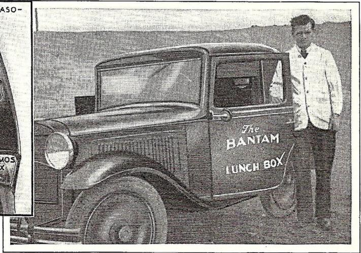
driver's seat, consists of a small 3-burner gasoline stove built across the rear inside, a small thermos ice box at the front, and sufficient shelves at sides and top to carry such edibles as bread, cheese, hot dogs, etc., as well as cooking and eating utensils. A small show case across the window sill displays cigarettes, candy, etc., at standard prices.
