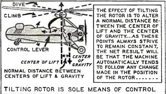
Drawing illustrates how tilting the rotor puts plane into a climb or dive. Tilting rotor to right or left banks the plane to right or left respectively. Lever is only control on ship.
