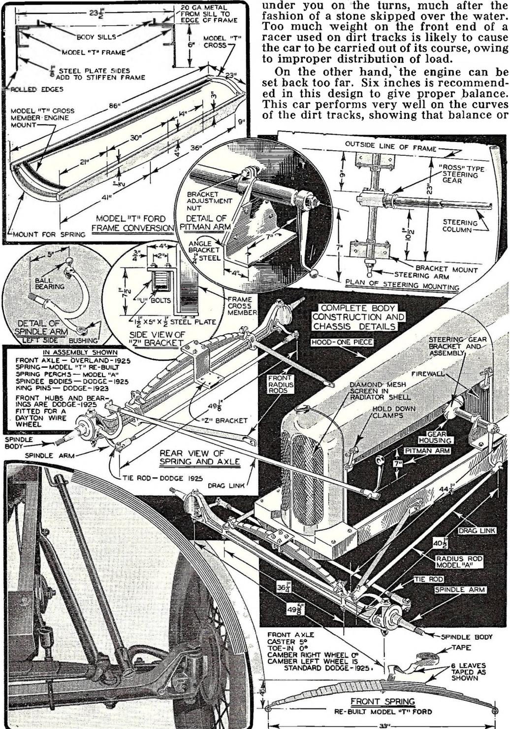
The tie-rod and radius rod hook-ups are shown in the photo immediately above. Front spring suspension, spindle arm details, and method of stiffening frame are shown in the drawings. Note the taped front spring, which is rebuilt.
