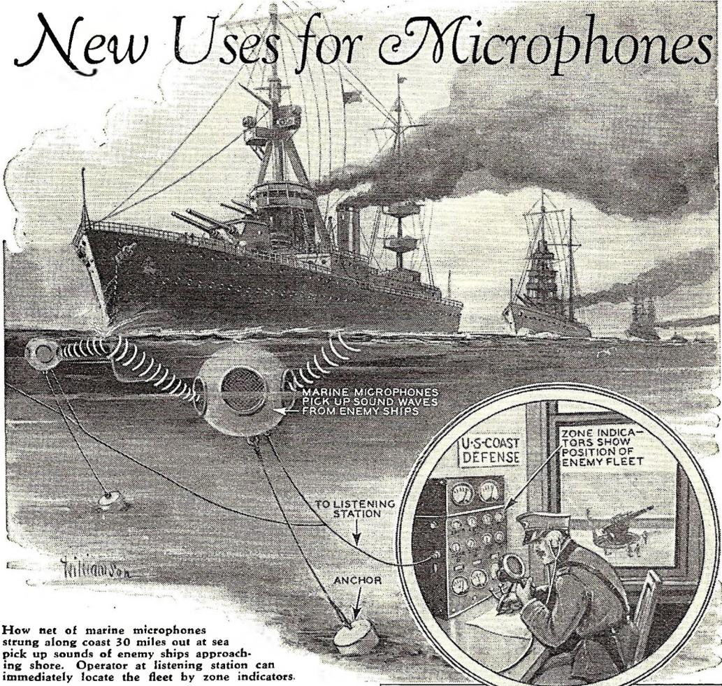
How net of marine microphones strung along coast 30 miles out at sea pick up sounds of enemy ships approaching shore. Operator at listening station can immediately locate the fleet by zone indicators.
