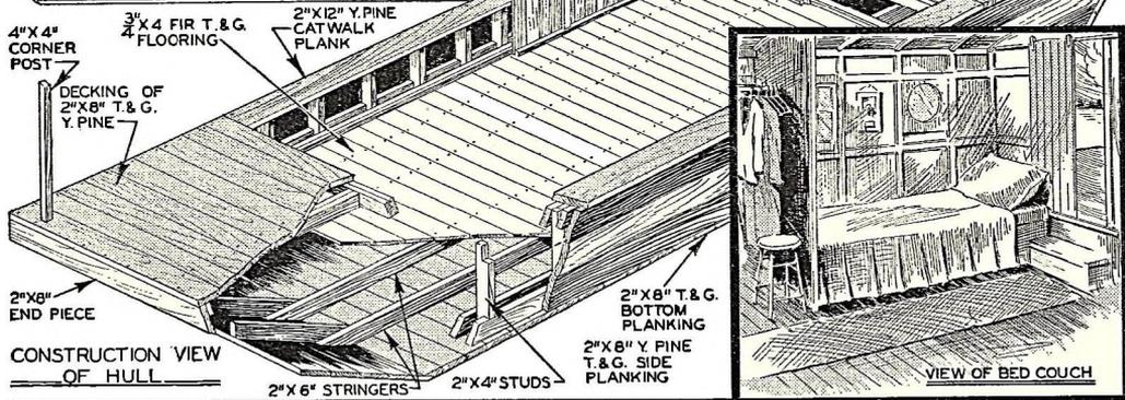
The size of the hull is 22 ft. long by 8 ft. 2 ins. beam, by 24 ins. deep. It will draw about five inches of water. The details of hull construction as explained in the text apply to the middle and half section views. Note the layout is the same as the M-M Cabinette Trailer. The cabin is the same as the one described in the trailer plans which ran in May issue.
