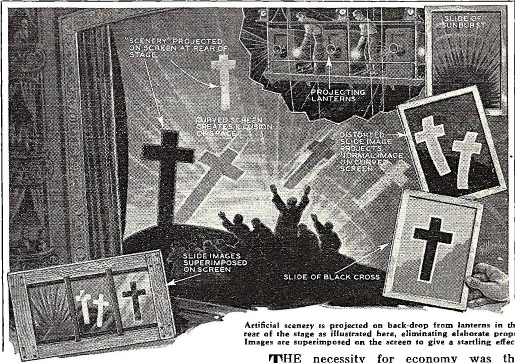
Artificial scenery is projected on back-drop from lanterns in the rear of the stage as illustrated here, eliminating elaborate props. Images are superimposed on the screen to give a startling effect.
