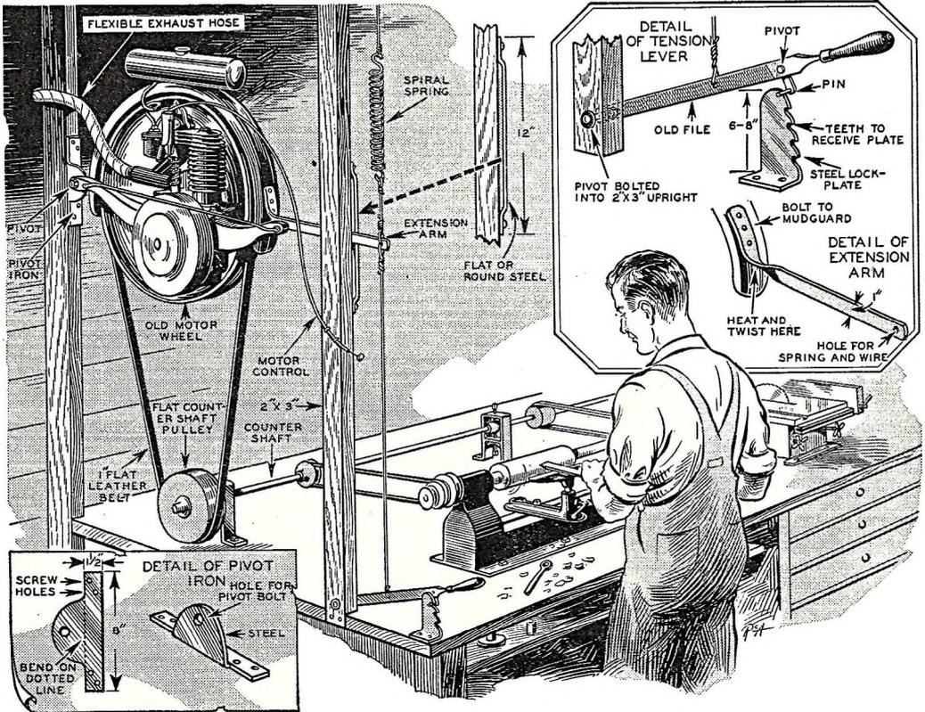
Motor wheel attaches to wall by means of a pivot iron as shown. Throwing down tension lever disengages belt, allowing motor to idle, while letting up on lever sets machine to turning. Fan on motor shaft will prevent overheating.
