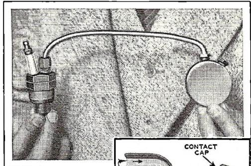
Above is seen the new self-cleaning sparkplug ready for installation. Drawing at right illustrates construction and operation. Feed pipe passes a small amount of gas into the chamber before each spark. Constant ignition of this gas keeps the interior clean and prevents accumulation of carbon.
