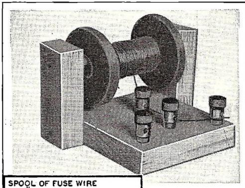
Whenever line is overloaded in experiment, the fuse wire between the two binding posts goes blooie. All you have to do then to install new fuse is pull wire through binding post holes, as shown.
