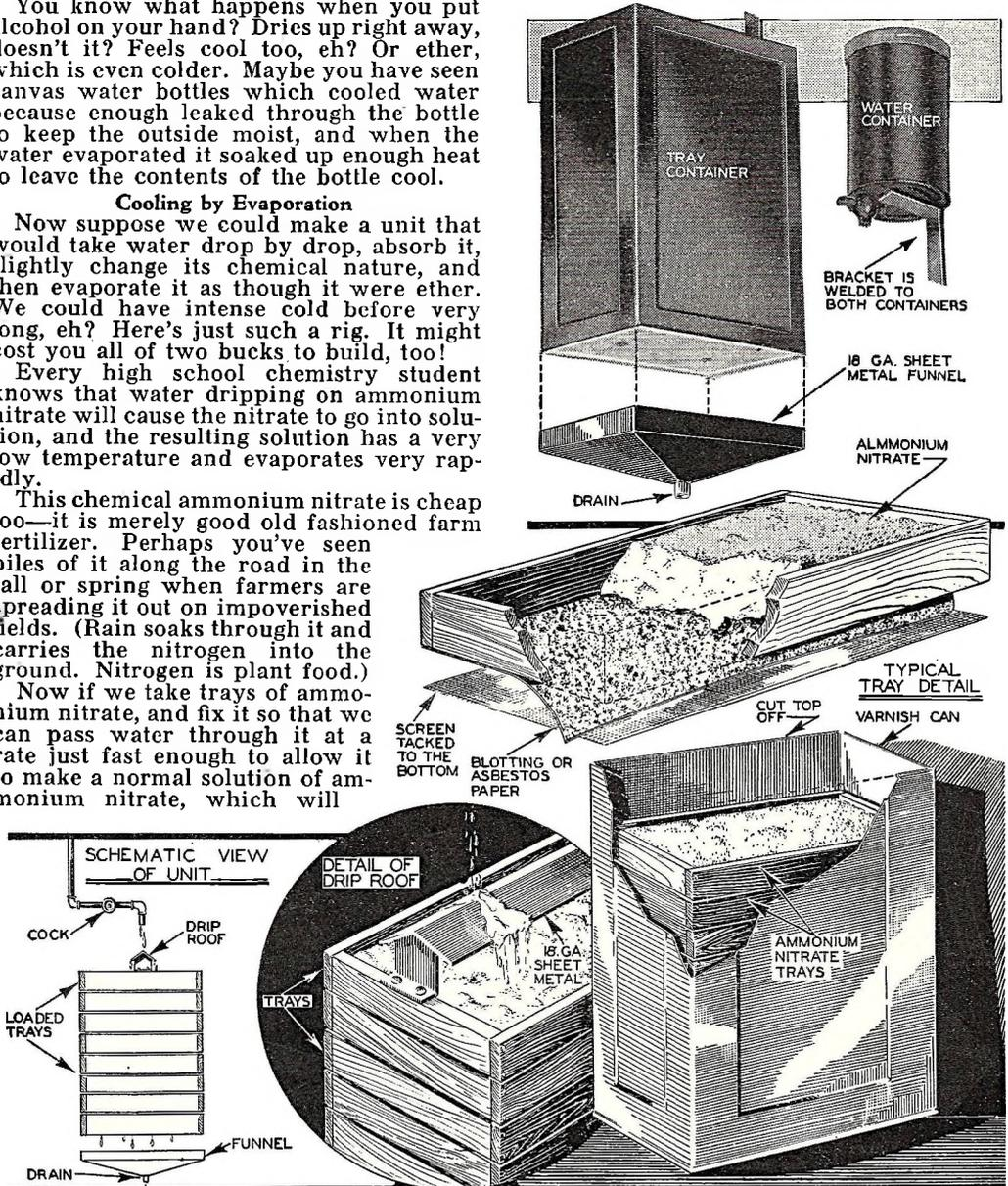
The drain must be used to pipe off the solution which results when the water drips onto the ammonium nitrate. A drip cock trickling water on a tin roof evenly distributes the water through the top tray, whence it filters to the others.
