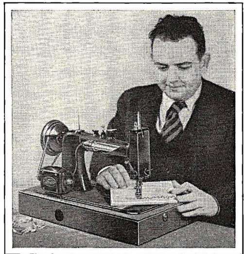
Attachment for sewing machine converts it into jig saw to cut out jig-saw puzzles. Handles wood up to  $\frac{3}{4}$ " thickness.
