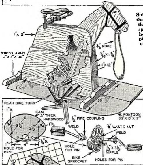
Five miles per hour is speed a good rider can make with this sea horse. Bike parts form the driving mechanism.
