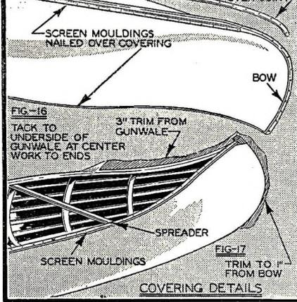
Working from the center at the keel the canvas is tacked down at the edges and stretched with a pair of pliers as it is nailed. One works towards the ends. Mouldings are then put on over the seams and the tacks before final finishing. Marine glue such as Jeffery's "C" quality or Casco casein glue will form good adhesives for the canvas.
