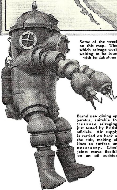
Brand new diving apparatus, suitable for treasure salvaging, just tested by British officials. Air supply is carried on back of the suit, making air lines to surface unnecessary. Limb joints move flexibly on an oil cushion.
