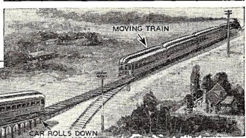
Launched with precise timing, the coach rolls down into main line just at right moment to hook onto the speeding train.
