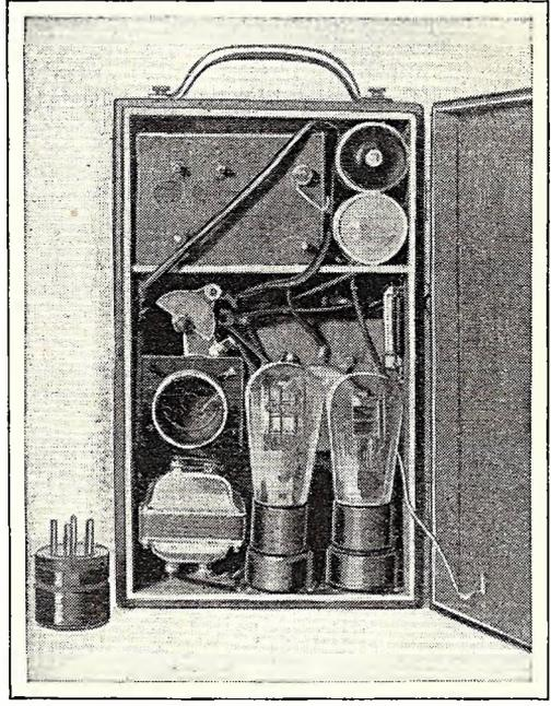
Arrange parts in cigar box as illustrated in this photo. COPPER SCREEN WIRE INSIDE COVER
