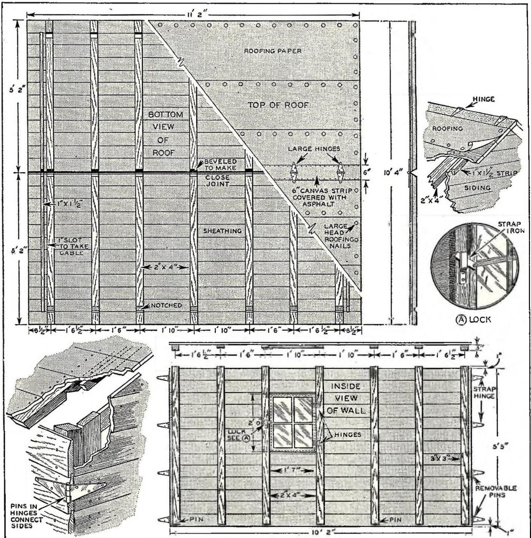
Plans for top and sides. Roof has notches in rafters to join with studding in the sides. Join hinges with pin to hold sides.
