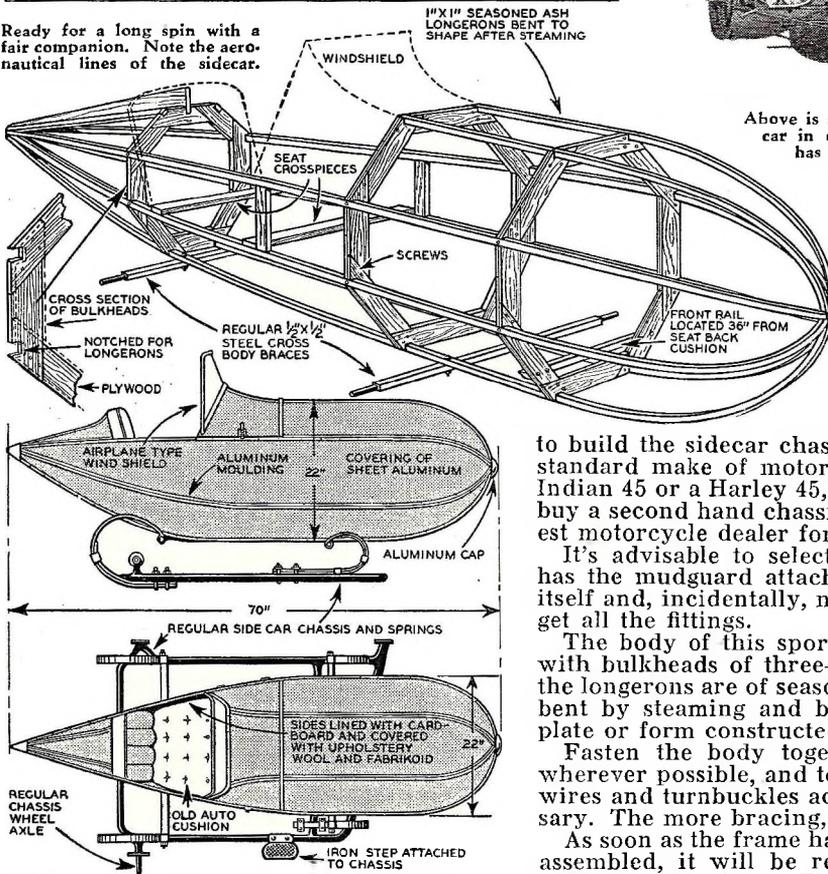
Drawing shows how sidecar body is mounted on two cross members of chassis, which can be obtained from any second hand dealer for a few dollars, if you're a good bargainer.
