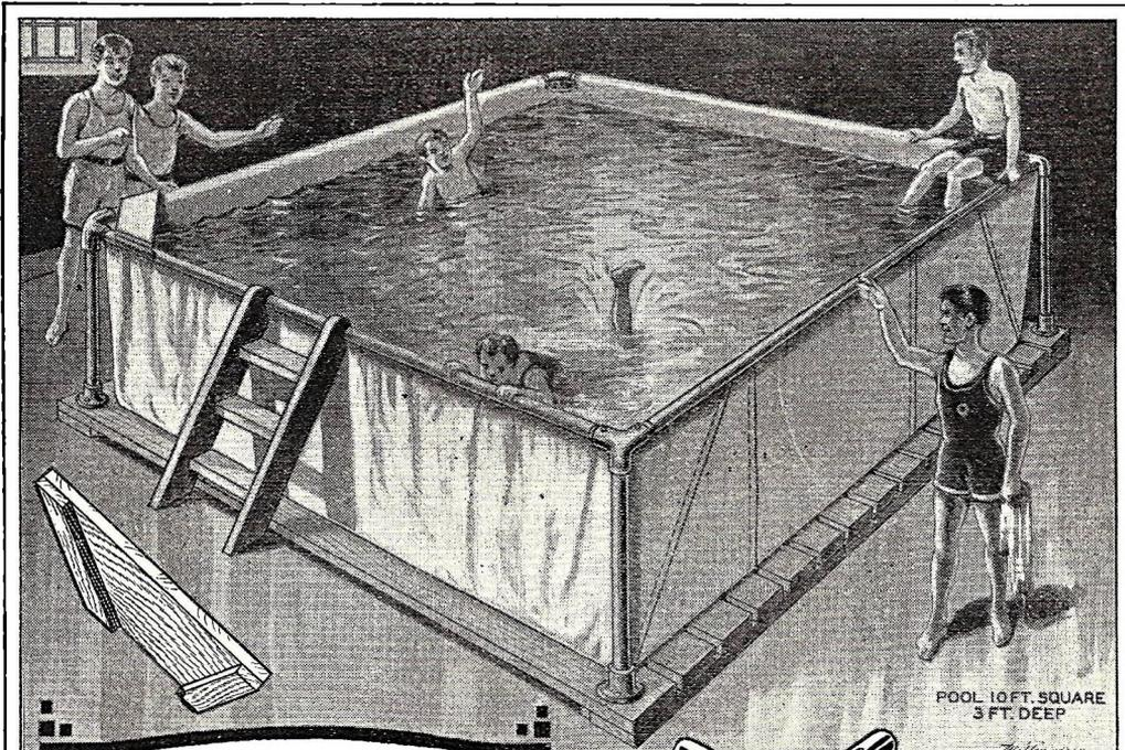
**T**HIS portable bathing pool for children is designed so that it can be set up anywhere without damage to the lawn, or taken down easily and stored in small space. The tank itself is three ft. deep and ten ft. square, made of brown waterproof canvas sewn with double seams and folded at ends, as shown. A wide hem is sewn on each side for the pipe supports and there is a reinforcing gusset in each corner.
