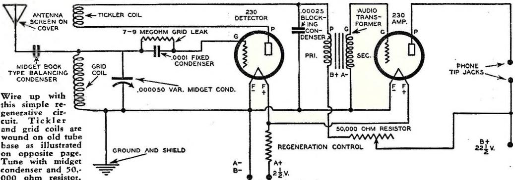
Wire up with this simple regenerative circuit. Tickler and grid coils are wound on old tube base as illustrated on opposite page. Tune with midget condenser and 50,000 ohm resistor.
