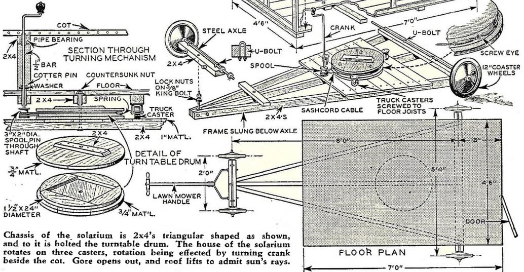
Chassis of the solarium is 2x4's triangular shaped as shown, and to it is bolted the turntable drum. The house of the solarium rotates on three casters, rotation being effected by turning crank beside the cot. Gore opens out, and roof lifts to admit sun's rays.
