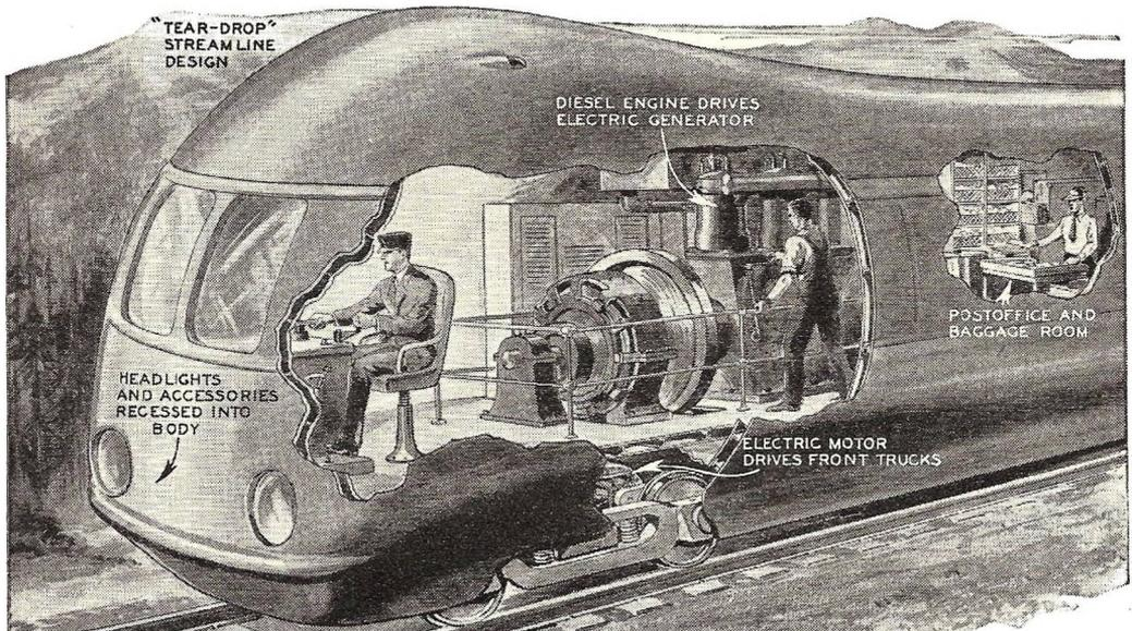
Features of carefully streamlined train under construction for Union Pacific Railway are given in drawing. Note clean, cinderless power mechanism—Diesel engine hooked to generator and motor on front trucks. At left, three-car streamlined train weighs no more than ordinary Pullman.
