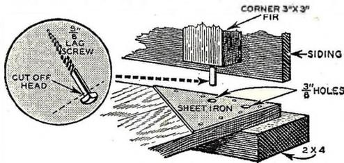
Assemble elements of floor and side as shown then cut down middle to form two hinged halves. Lag screws in side are set in  $\frac{3}{8}$  in. holes in floor to hold house in place.
