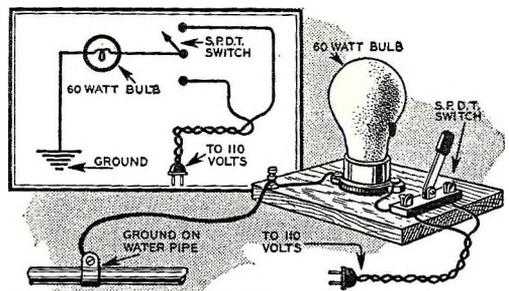
Mount parts of tester on baseboard and wire up as shown.
