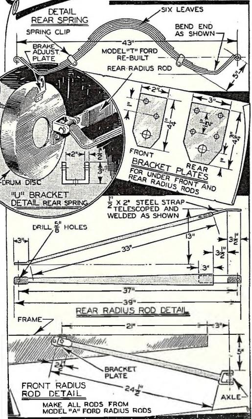
Immediately above are shown the dimensions of the front and rear radius rod installations. These are all made from Ford model "A" radius rods.
