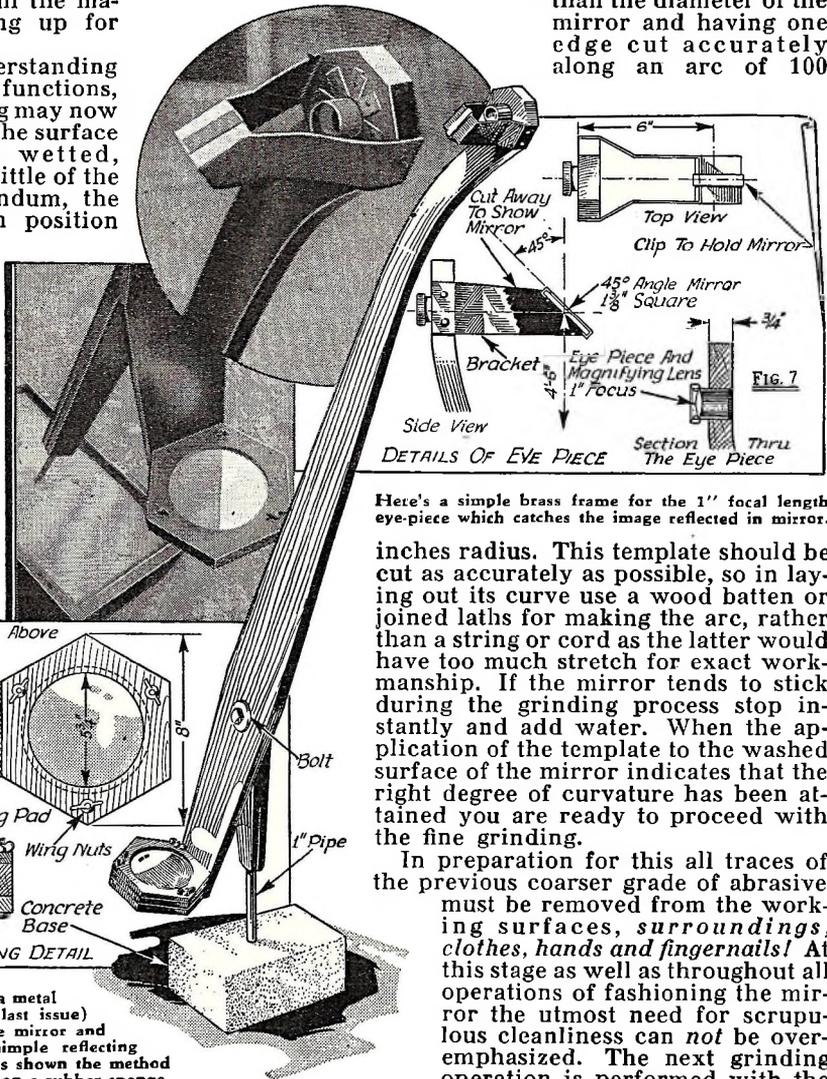
Here's a simple brass frame for the 1" focal length eye-piece which catches the image reflected in mirror.
