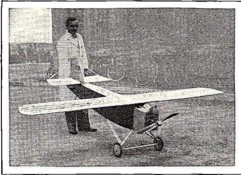
Much experimenting is being done with miniature gas powered airplanes that really fly. Here is one built by Juniors of the Pasadena Technical High School. One horsepower.
