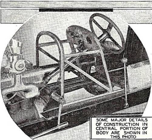
The steering wheel is set just off the center line, as shown above and in the top right drawing, opposite page. The placing of Pitman rod and body frames is also shown here.
