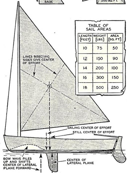
Above are shown a few of the more commonly used sail rigs. The area of a triangle is  $\frac{1}{2}$  base times the altitude. Below is explained the reason that the center of effort of the sail must be placed slightly ahead of the center of lateral resistance when still. The lateral center travels forward faster than the center of the sail. Both must balance, or nearly so to give proper sailing ardency, or tendency to come up into the wind with a free tiller.
