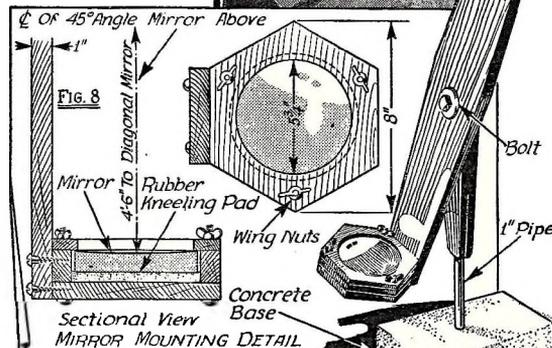
Either a wood frame or a metal pipe frame (as shown last issue) can be used to hold the mirror and the eye-piece of the simple reflecting type telescope. Above is shown the method of mounting the mirror on a rubber sponge.
