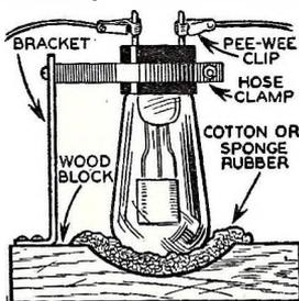
Hook tube into circuit with wires leading from the clip on prongs.
