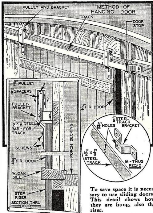
To save space it is necessary to use sliding doors. This detail shows how they are hung, also the riser.
