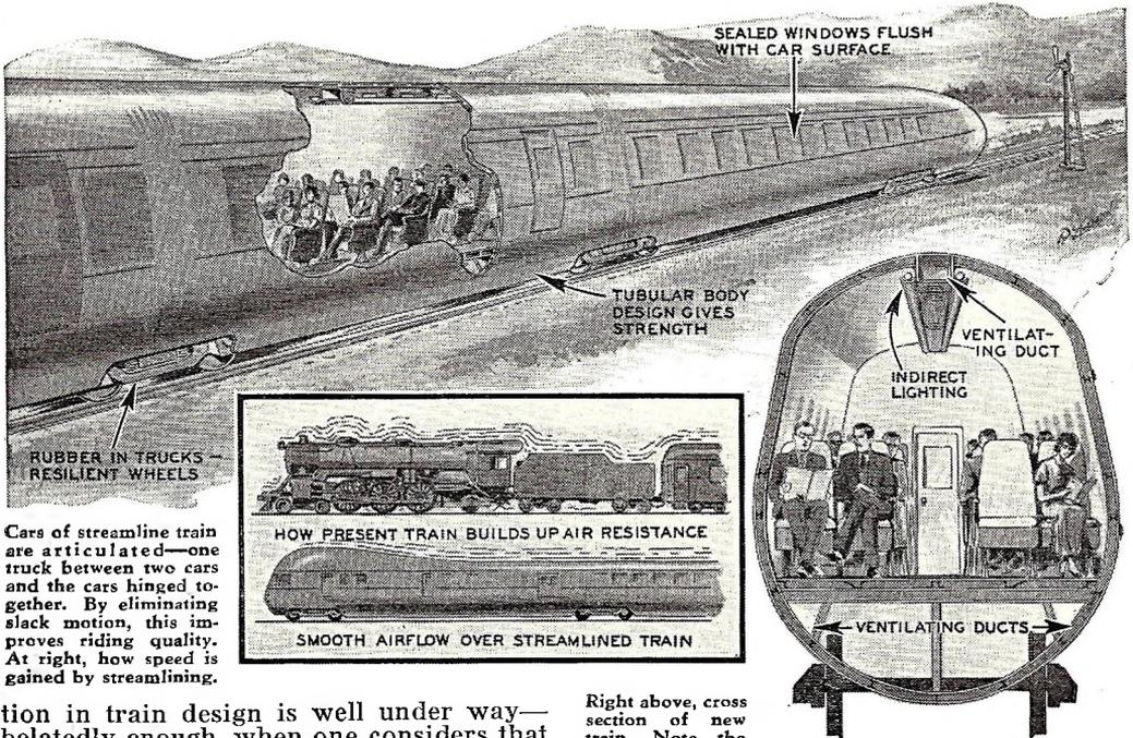
Cars of streamline train are articulated—one truck between two cars and the cars hinged together. By eliminating slack motion, this improves riding quality. At right, how speed is gained by streamlining.
