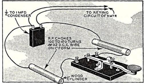
Transmitter "thumping" is reduced to minimum with this filter, which is hooked into the key circuit as shown here. Use condenser having rating of double plate voltage.
