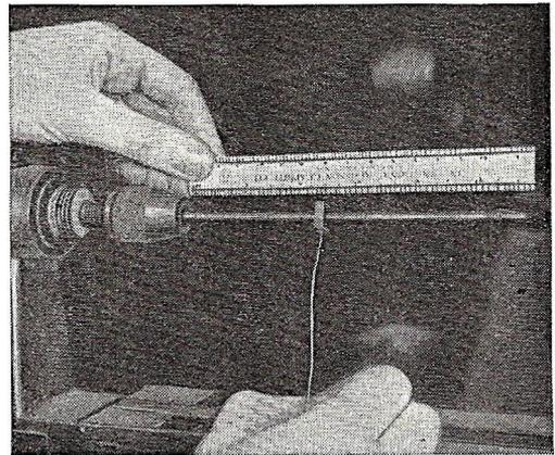
Speed is determined from calculations involving length the nut travels and the number of threads to inch on the rod. Time revolutions with stop watch for most accurate results.
