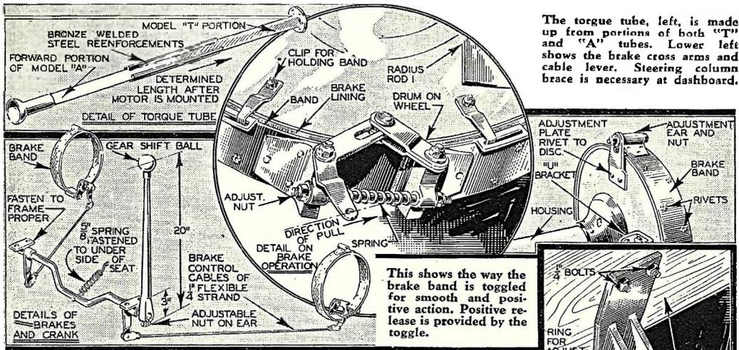
The torque tube, left, is made up from portions of both "T" and "A" tubes. Lower left shows the brake cross arms and cable lever. Steering column brace is necessary at dashboard.
