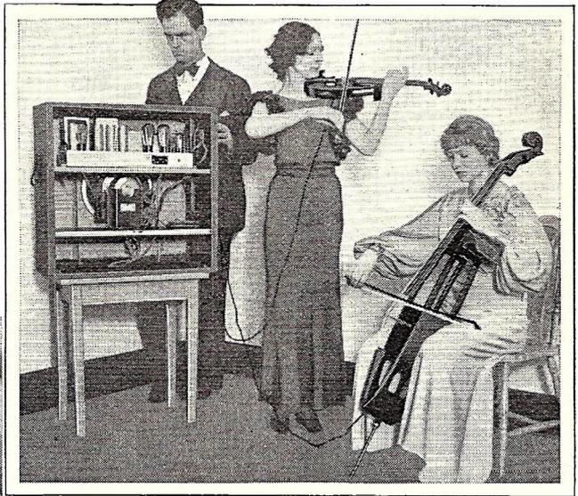
A recital being given with one of the new violins and cellos. Output of the pick-up is here seen utilizing amplifier and speaker of ordinary home radio set for reproduction. Volume from violin fills auditorium.
