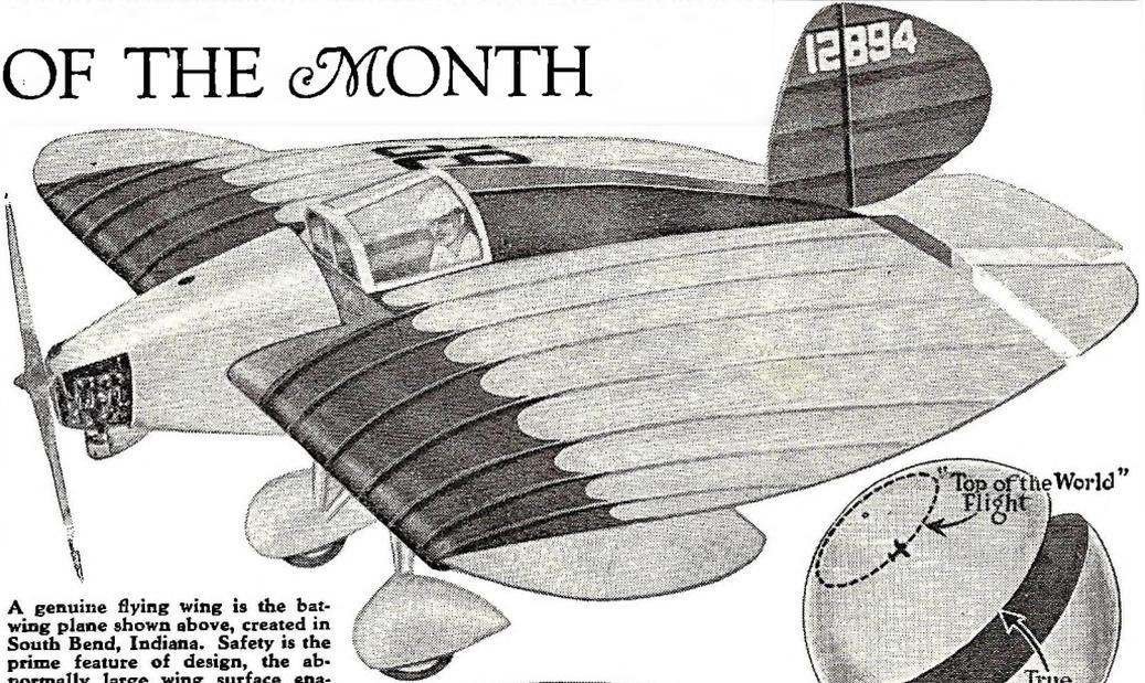
A genuine flying wing is the batwing plane shown above, created in South Bend, Indiana. Safety is the prime feature of design, the abnormally large wing surface enabling ship to descend nine feet a second, a gentle speed comparable to that of a chute jumper.
