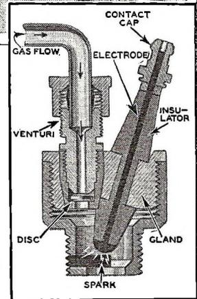
**A** NEW sparkplug now on the market is said to be self-cleaning and to outwear the automobile in which it is installed. The feed pipe passes a very small amount of gas into the chamber before each spark. The constant ignition of this gas keeps the interior thoroughly clean and prevents the accumulation of carbon.
