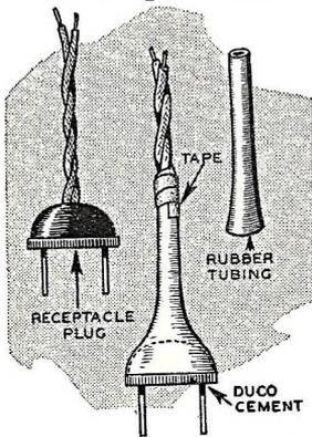
Rubber tubing is slipped over the wire and glued to the plug.
