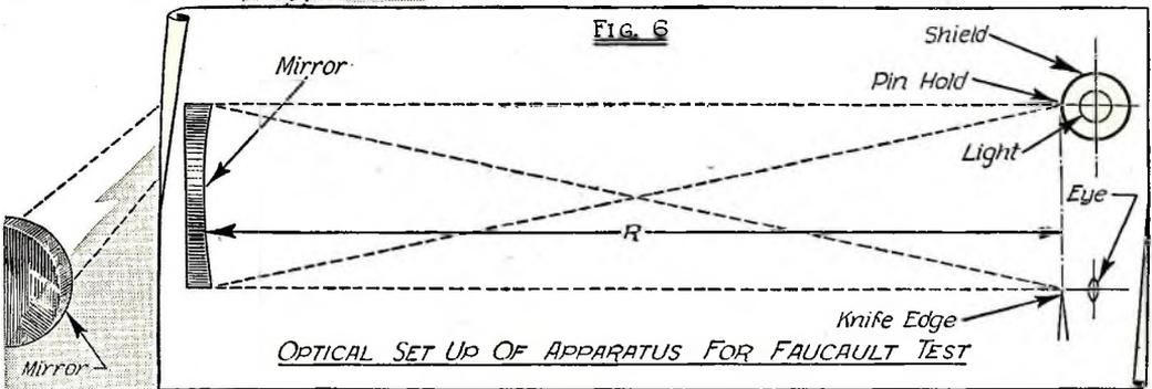
Above is shown the diagram of the Foucault test. If the mirror is truly spherical the pin point of light emanating from the tinfoil will appear to the eye as a bright flat surface throughout the face of the mirror.
