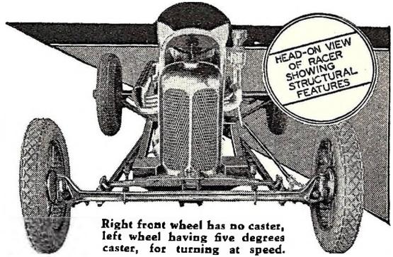
Right front wheel has no caster, left wheel having five degrees caster, for turning at speed.
