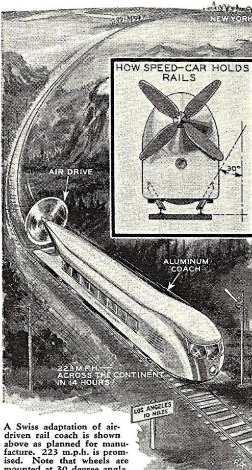
A Swiss adaptation of air-driven rail coach is shown above as planned for manufacture. 223 m.p.h. is promised. Note that wheels are mounted at 30 degree angle.
