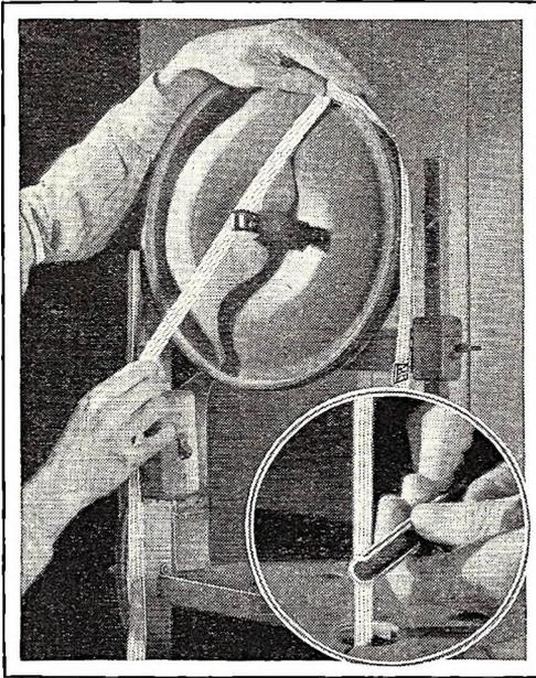
Twilled tape is fitted over discs in place of regular band saw as illustrated in photo above. Articles to be polished are held against the tape as demonstrated in the inset.
